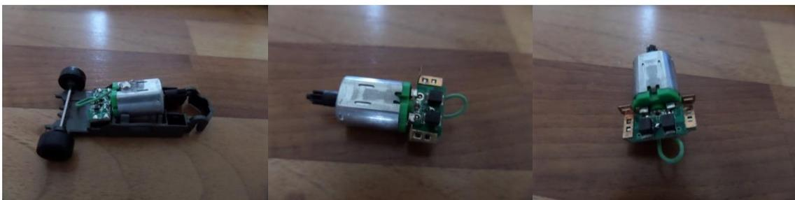
The circuit board is attached to the motor by a soldered joint to the motor tabs. The circuit board has the hangers for the pickups again, soldered to it. Pickup springs sit on this hanger and this creates a second electrical path from the pickups. **Removal of the wire is possible by cutting or desoldering, and the motor still runs.**
