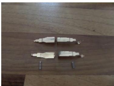
Guide pin: This is positioned in a much more forward position, ahead of the front axle. The length is approx the same as the old ones. Consistency in the length of the older MG guide pin length was always questionable. The 3 MG+ I have to hand all appear to be the same. It appears to be a different batch to the older car as these do not have a Pip on them.
