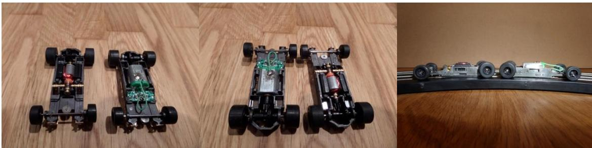
Rear axle: The rear axle is clipped into the chassis and has a 22?? tooth gear. The gear saver now spans the width of the rear cutout. The gear appears to run true. The hubs do seem to run slightly off. The axle is well clipped in and the chassis has a cutout so the axle can only be put in one way. The rear gear meshes with a 7 tooth pinion. This pinion is now a long pinion along the length of the motor shaft. The mesh feels very smooth with no notchiness.
