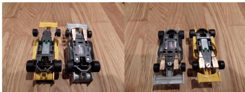
The body unclips from the chassis which is a snug and secure fit. The motor can now be seen to have a small circuit board in front of it with a wire being attached to the topside of the motor. This board is largely down to reducing electronic interference. The chassis height with the can motor is the same as the older chassis.
