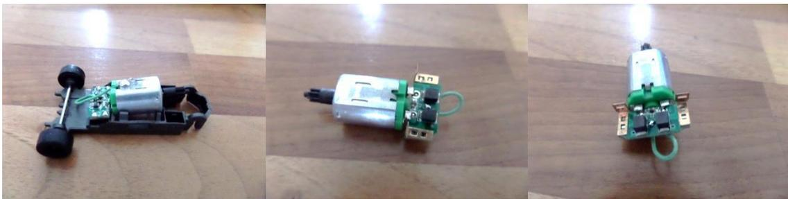
The circuit board is attached to the motor by a soldered joint to the motor tabs. The circuit board has the hangars for the pickups again, soldered to it. Pickup springs sit on this hanger and this creates a second electrical path from the Pickups. Removal of the wire is possible by cutting or de-soldering, and the motor still runs.
